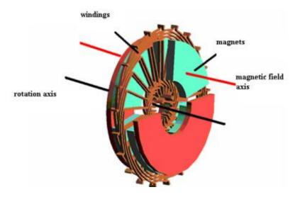
Figure 5 Axial flux brushless dc motors
