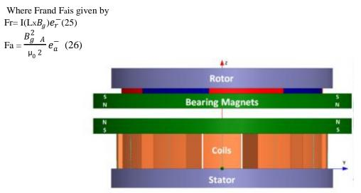
Fig.7. Magnetic levitated design of BLDC Motor (Courtesy: Prof.Ahmet FENERCIOG LU)
