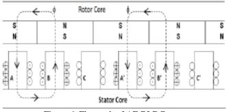
Figure 6. Flux path of AF-BLDC motor
